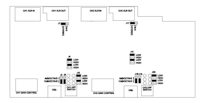
Figure 3. Circuit Board Jumper Locations SN #V054 and below
